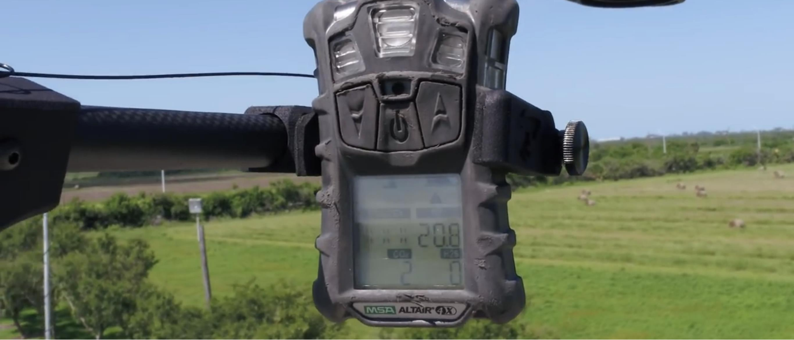
Hazmat Sampling From Drone
